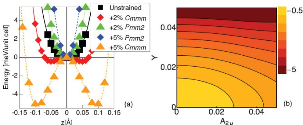
FIG. 3. (Color online) (a) Total-energy change for static atomic displacements along the  $A_{2u}$  mode under uniaxial (110) strain for atomic positions relaxed with imposed  $Cmmm/Pmm2$  symmetry. Here, only the second symmetry class allows for polarization in (110) direction. (b) Energy landscape for mixed displacements along  $Y_0$  and  $A_{2u}$  for 2% tensile strain in (110) direction.
