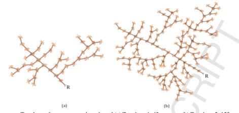
Figure 9. Topology of neuron network evaluated (a) Topology 1, 43 neurons, (b) Topology 2, 153 neurons
