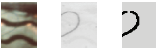
Fig. 1. From left: Original patch, infrared (IR) scan and SDIp detected binary mask. Note how the IR scan shows the level of transparency, and that the SDIp detector overdetects the limit of the blotch.
