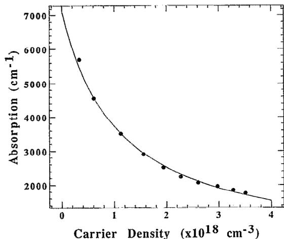
FIG. 3. Saturation of heavy hole exciton absorption line in GaAs/ $\text{Al}_{0.3}\text{Ga}_{0.7}\text{As}$  multiple quantum well. The dots are experimentally obtained from reflectivities of the asymmetric Fabry–Perot resonance; the solid line is a theoretical fit using a simple absorption saturation model.
