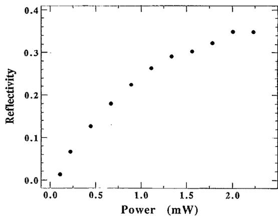
FIG. 2. Reflectivity of asymmetric Fabry-Perot étalon, at the resonance wavelength of 850 nm, as a function of incident power.
