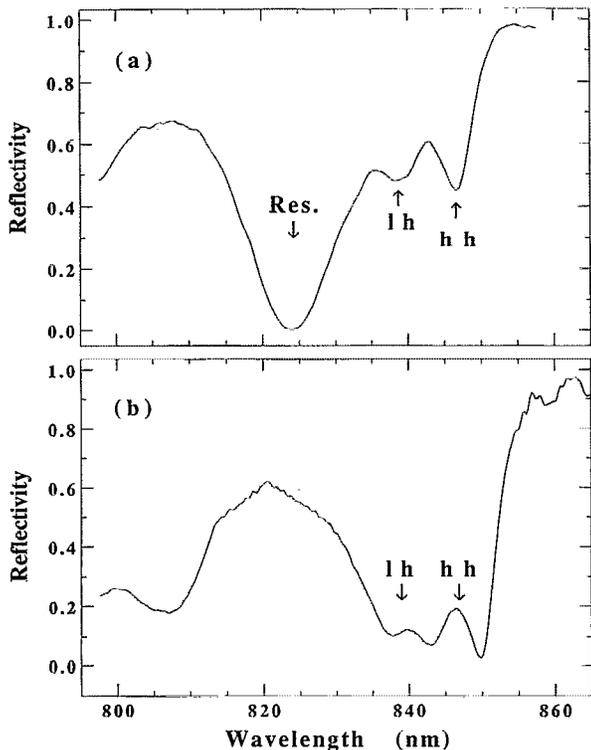
FIG. 1. Reflectivity of asymmetric Fabry-Perot étalon as a function of wavelength at two different sample positions (a) and (b). The light hole (lh) and heavy hole (hh) excitons are clearly resolved in (a) and the Fabry-Perot resonance (Res.) can be seen to shift spectrally due to small changes in cavity dimensions from (a) to (b).
