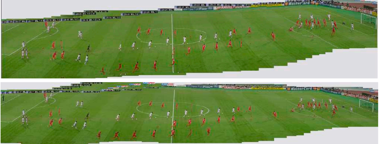
Fig. 4. Mosaics of the football sequence. Top mosaic: using non-parametric method only. In this mosaic as the camera to the right the top sideline tends to curve upwards in the mosaic; Bottom Mosaic: using the hybrid algorithm.
