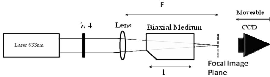
**Figure 4:** To form non diverging Bessel beams a lens is places at its focal length away from the focal image plane above.
