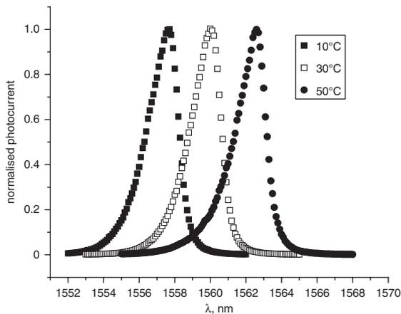
Fig. 1 Wavelength response of microcavity against temperatures, for three temperatures
