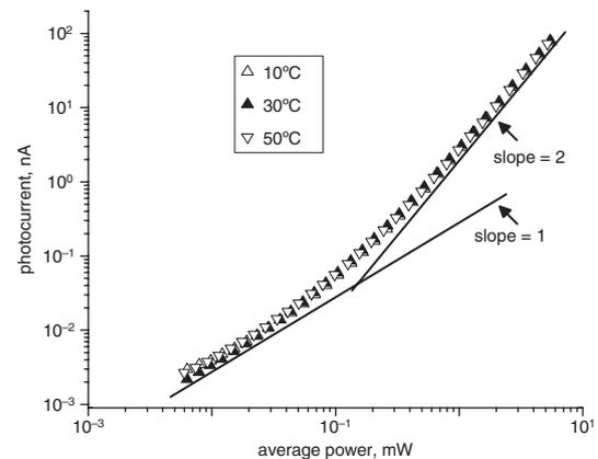
Fig. 3 Photocurrent against incident power for different temperatures
