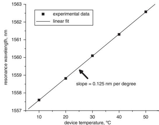
Fig. 2 Microcavity resonance wavelength against temperature
