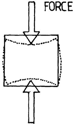
Fig. 5. View of the cavity cross section under a load.
