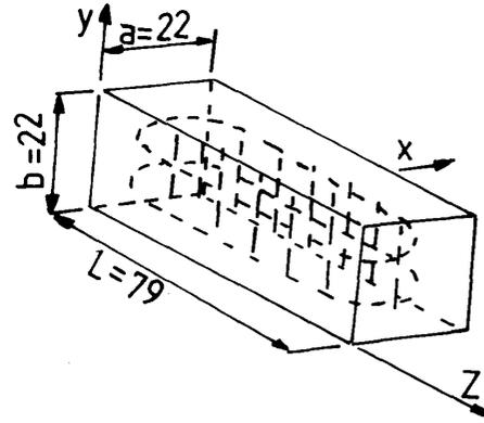
Fig. 2. Cavity resonator with  $H_{101}$  modes.
