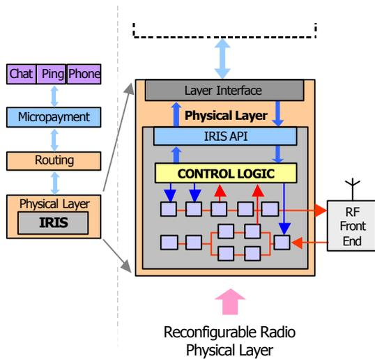
Figure 5: Spectrum Rental – linking the higher layers with the Reconfigurable Radio
