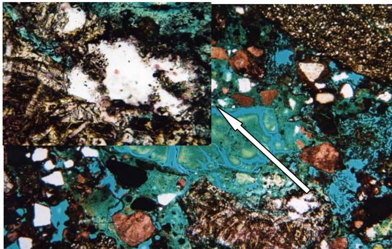
Figure 8 - Amorphous and crystalline hydrates formed in a pozzolanic aggregate (a fragment of crystalline rock, probably a dolerite). Top left insert shows detail of the pozzolanic reaction. St John's Bridge pier core, destroyed by the 1763 flood. Field of view 4.2mm. Parallel polars.
