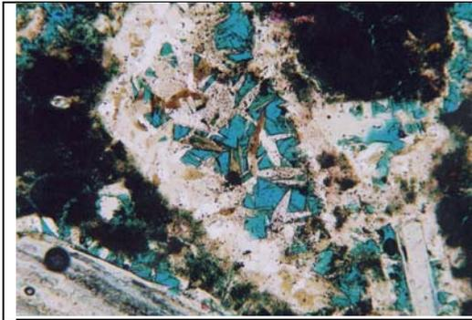
Figure 10- Gypsum originating from atmospheric pollution in a lime mortar pointing Dublin's Medieval City wall. 10X. Polarised light.
