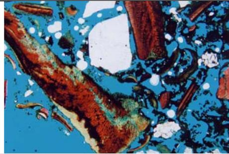
Figure 8- Lime binder loss through calcite dissolution: St Mary's Church Youghal, County Cork. 2X parallel light.
