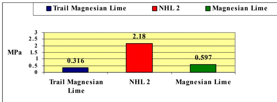
Figure 7- Compressive strength of natural, feebly-hydraulic lime (NHL 2) and magnesian lime mortars correctly mixed and incorporating an excess of water (Trail Magnesian Lime). (Average of 6 samples).
