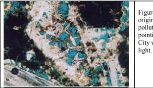
Figure 10- Gypsum originating from atmospheric pollution in a lime mortar pointing Dublin's Medieval City wall. 10X. Polarised light.
