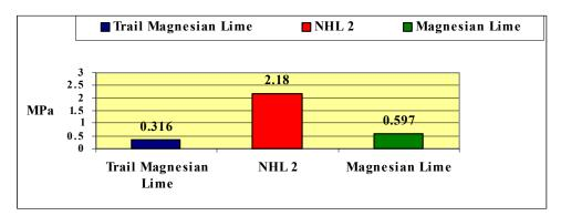
Figure 7- Compressive strength of natural, fleebly-hydraulic lime (NHL 2) and magnesian lime mortars correctly mixed and incorporating an excess of water (Trail Magnesian Lime). (Average of 6 samples).
