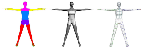
Figure 2: (a) material IDs assigned to mesh, (b) mesh with greyscaled textures and diffuse colours set to white, (c) mesh with skeleton fitted.
