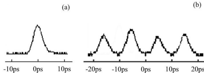
**Figure 2: Real-Time TPA Sampling Measurement of (a) 10GHz Optical Pulse; (b) 100Gbit/s Pulse Train**
