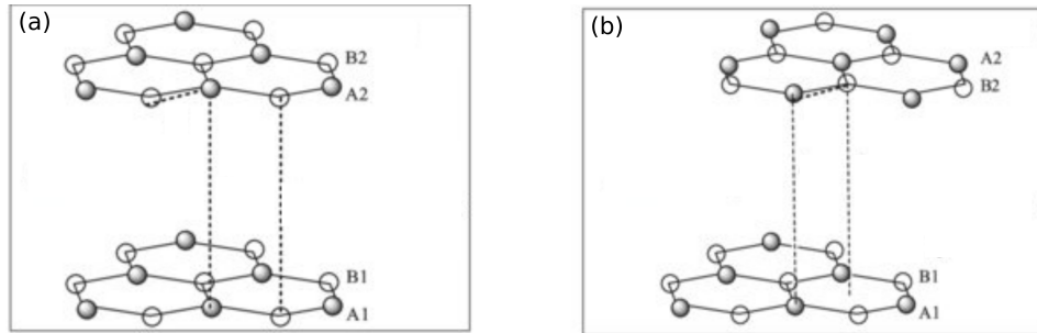
Figure 2.2: Interlayer interactions for (a) AA-stacked and (b) AB-stacked BLG. Figures (a) and (b) adapted from [127].
