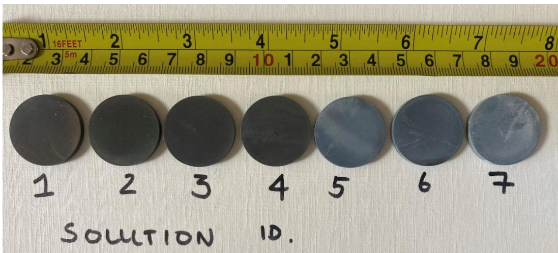
Figure 2.3: Photograph of HA samples on Ti coupons as deposited by Solutions 1-7.
