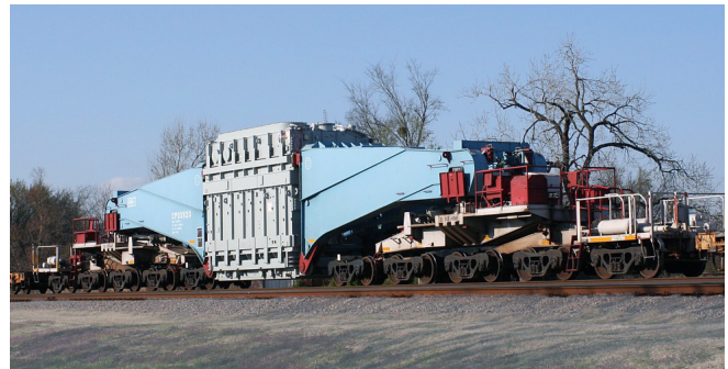
Figure 1: A 20-axle freight wagon for transport of an electrical transformer.
