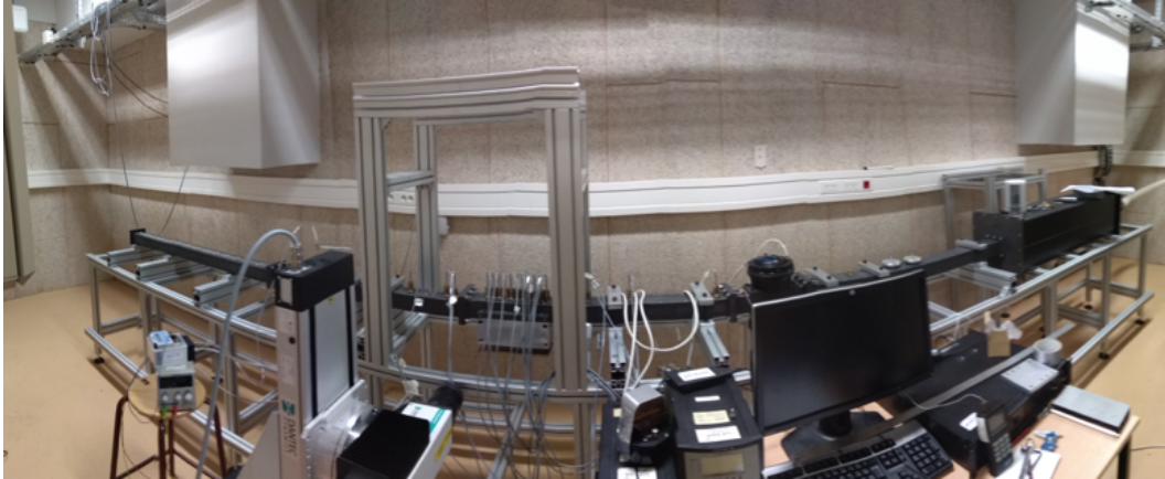
Figure 3.4: Photo of the Optical Duct located in LAUM [164]. The acoustic source is located upstream of the test section, on the right-hand side of the image.
