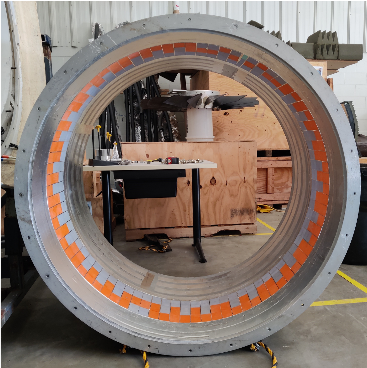
Figure 7.11: Completed liner installation in the casing prior to being attached to the ANCF.
