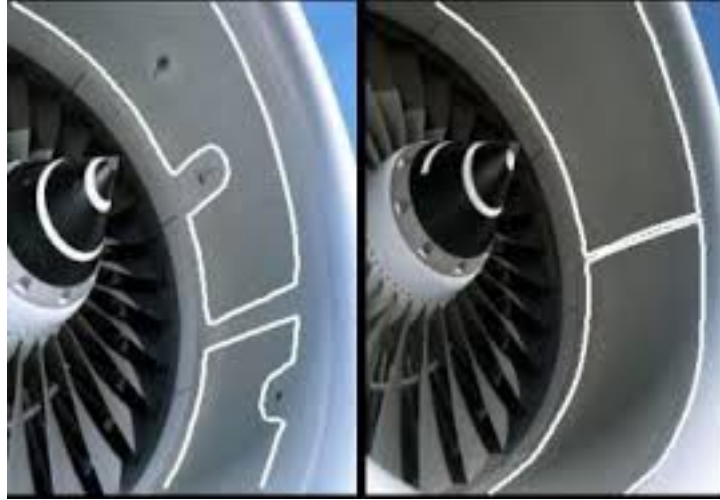
Figure 2.10: Representation of the size of the acoustic liner splice between two generations of engine liners [78].
