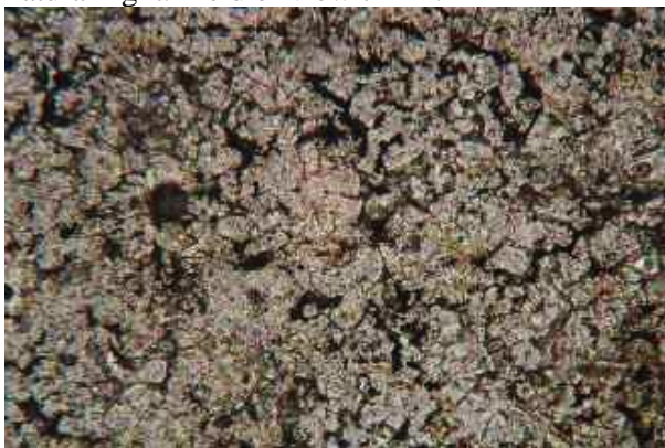
Fig.4. Detail of hydraulic calcium silicates in an iron interphase. 20X natural light. Field of view 0.7 mm.
