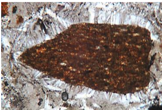
Fig.16. Detail of secondary fibrous gypsum filling the interface around aggregate. 10X, polarised light. 1.42 mm.
