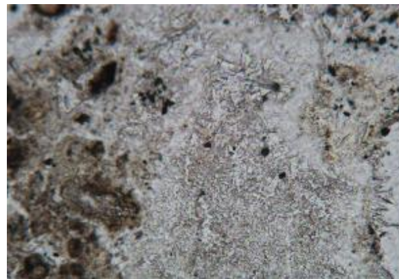
Fig.5. Plaster A. Abundant microcrystalline gypsum (white) in the binder. 10X. Natural light.
