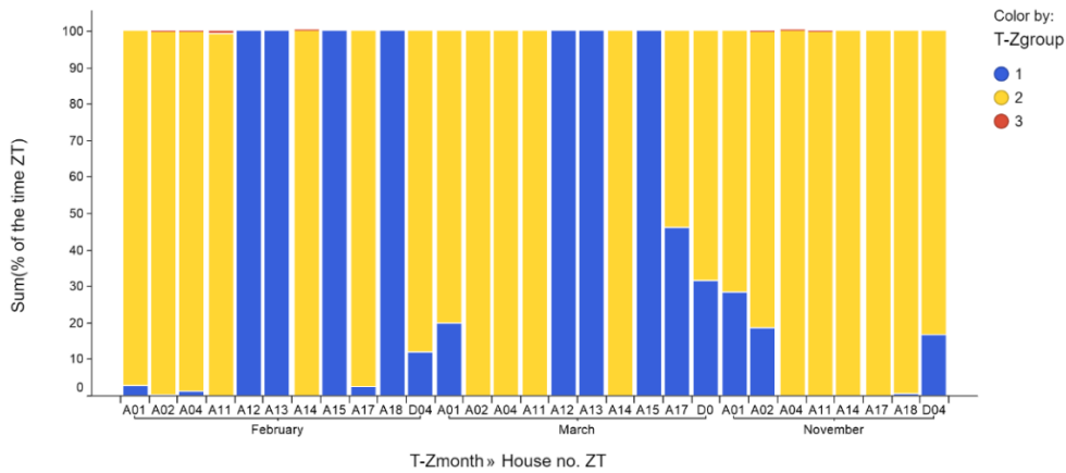
Figure 7.1 Temperature exceedances in the living/kitchen area; T = 18\text{-}25^{\circ}\text{C} (in yellow); T < 18^{\circ}\text{C} (in blue), and T > 25^{\circ}\text{C} (in red).
