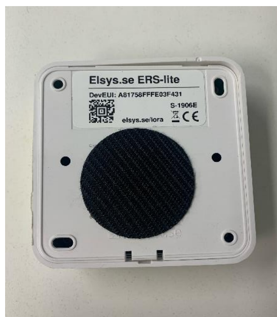
Figure 3.11 Strip tape for hanging sensors (black circle)
