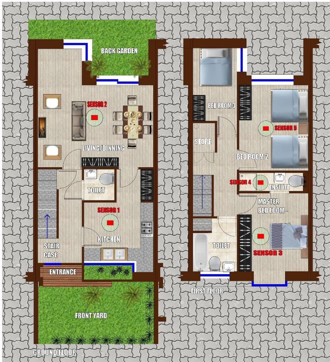
Figure 3.15 Drawing indicating the locations of the five sensors provided in each typical house
