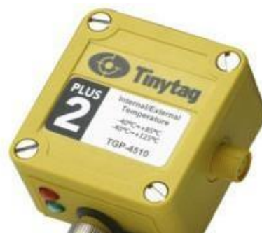
Figure 3.3 External T and RH monitor
