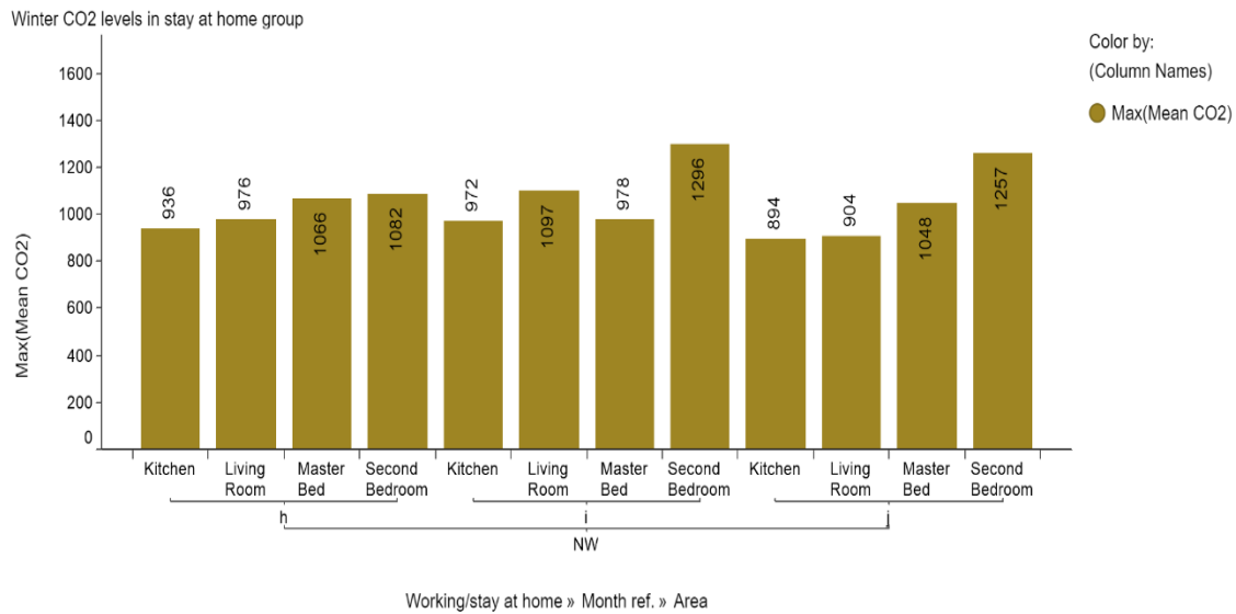
Figure 5.8 Average maximum monthly CO 2 levels in different zones of non-working families in Winter
