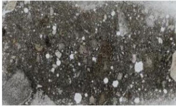
Figure 5-10 \text{Na}_2\text{SiO}_3 + \text{NaOH} activated GGBS cured at 60^\circ\text{C} shows stronger reaction, with a more homogeneous matrix where much of the GGBS has become cement.
