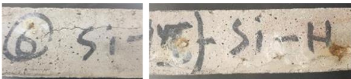
Figure 5-7 \text{Na}_2\text{SiO}_3 activated GGBS after 20 wet-dry cycles. Left image 20^\circ\text{C} cured, right 60^\circ\text{C} cured showing cracks, delamination and slight efflorescence.
