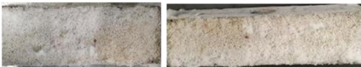
Figure 5-8 Efflorescence on NaOH activated GGBS after 20 freeze- thaw cycles (left 20°C-cured; right 60°C).
