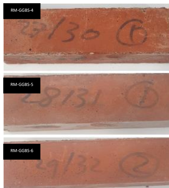
Figure 5-30 RM-GGBS-4, RM-GGBS-5 and RM-GGBS-6 undamaged after cycling.
