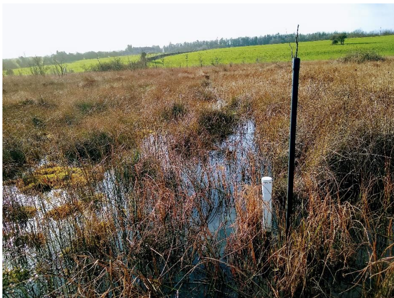
Figure 4.2. A phreatic tube (left) and piezometer (right) installed in Scragh Bog.
