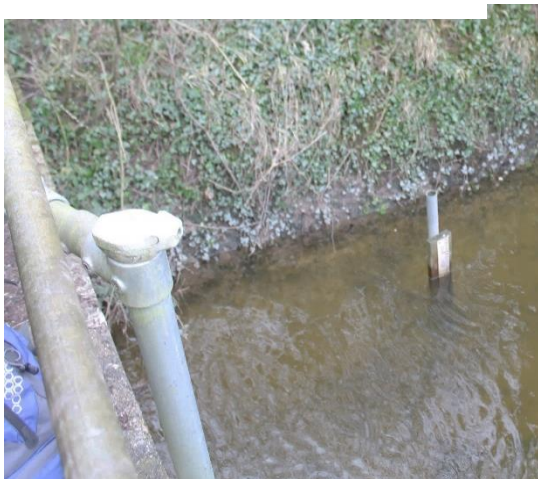
Figure 4.10. Tory Hill hydrometric station and staff gauge.
