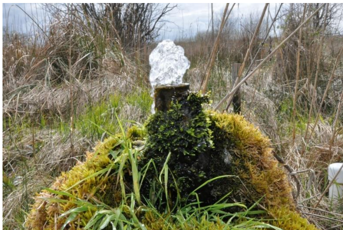
Figure 7.6. Artesian flow conditions in Pollardstown D. The mounds around the piezometer is tufa which is created by precipitation of carbonate minerals in the groundwater.
