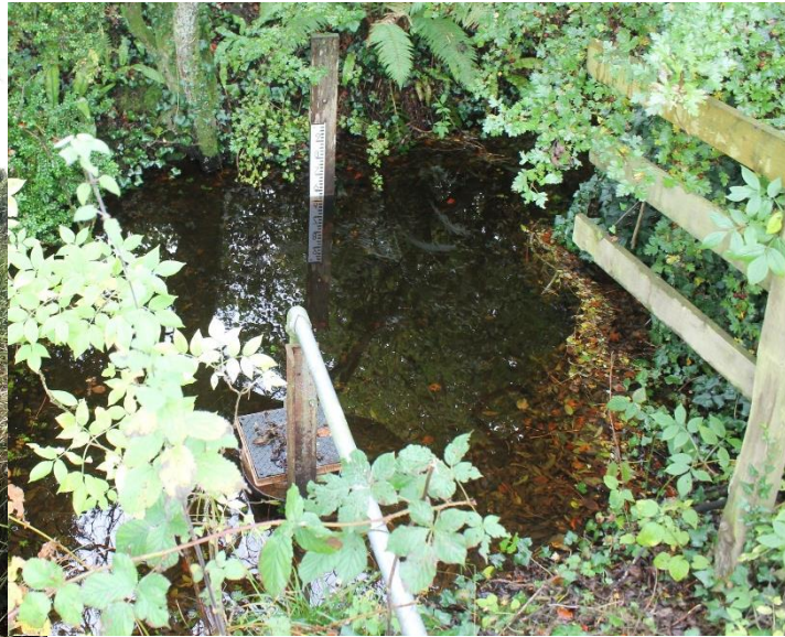
Figure 4.9. Scragh Bog hydrometric station and staff gauge.
