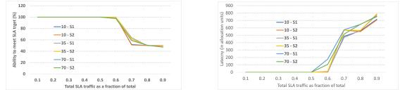
(a) Ability to meet SLA for varying amount of SLA traffic (b) Average delay (expressed in allocation unit of 0.11 µs each)
