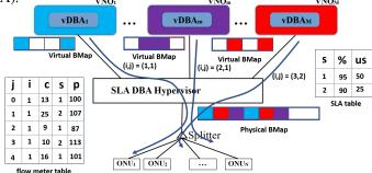
Fig. 1: Architecture of the SLA-oriented DBA hypervisor, implementing a stateful mechanism through meter tables.
