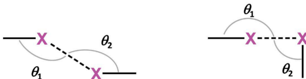
Fig. 2.7 Types of intermolecular halogen⋯halogen interactions, showing type I (left) where \theta_1 \approx \theta_2 and type II (right) where \theta_1 \approx 90^\circ and \theta_2 \approx 180^\circ . 61
