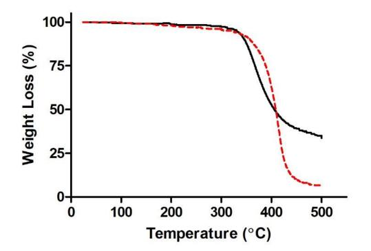
Thermogravimetric thermograms showing % weight loss at increasing temperatures of epoxy resins based on different ERMs in N2. DGEBA and PinoDGE. N=3.
