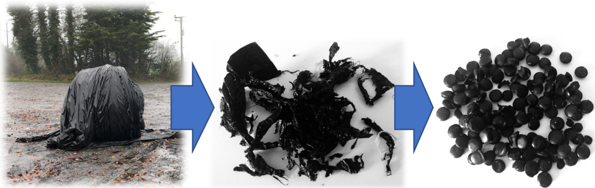
Plate 12.7 Plastic waste to reusable nurdles Industrial plastics are recycled in the new Littleton facility. Discarded rolls are cut up into smaller pieces before conversion into nurdles which can be repurposed into new plastic products.
