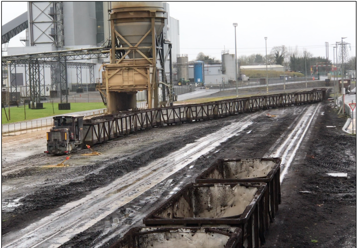
Plate 4.8 A Bord na Móna rake at ESB Lough Ree, Co. Longford A Bord na Móna locomotive, or ‘loco’, pulling wagons at the ESB Lough Ree power station, March 2020. A loco plus wagons (up to 16) is collectively known as a ‘rake’ (Clarke, 2010: 390).
