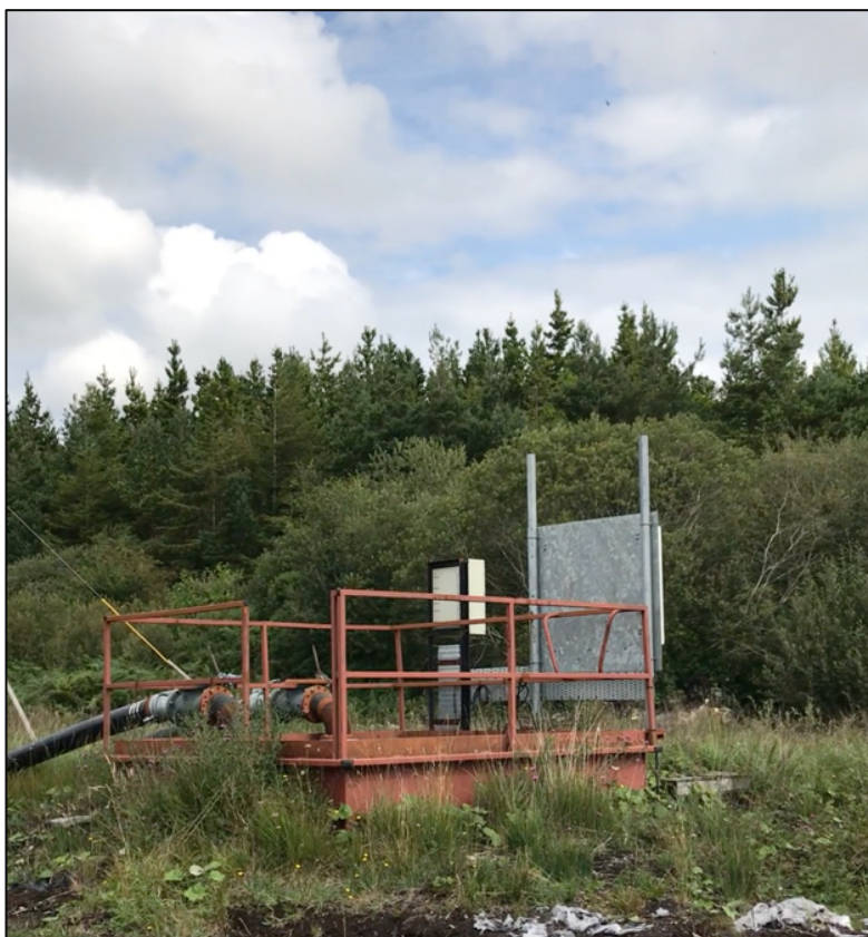
Plate 11.3 Bog pump at Carrickhill bog, Littleton, Co. Tipperary. It was used to drain water from the bog when it was in production.
