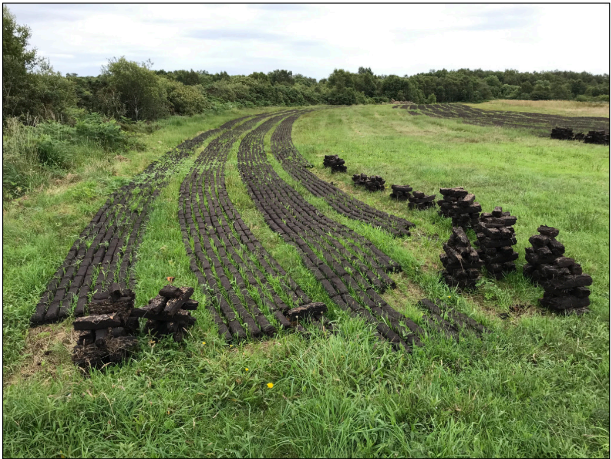
Plate 4.4 Extruded turf, Co. Longford Turf spread out, ready to be footed. Peat is mechanically cut from a bog face bank by a contractor using an excavator. It is mixed in a hopper before it is extruded onto adjacent ground. It is then manually ‘footed’ by its owner so that it can dry out. Once the turf is ready it is transported home.
