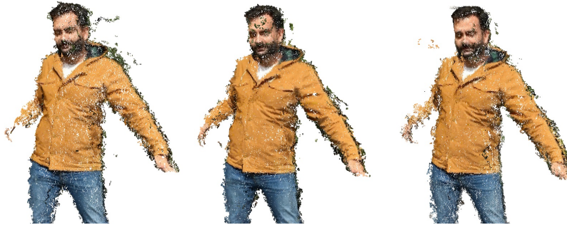
Figure 1.4: Filtering Point Cloud Sequences. An incoherent point cloud sequence typical of a modern sparse VV system such as that of Pagés et al. [3]. Notice in particular the structure noise patches around the head.
