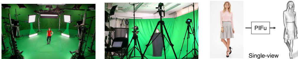
Figure 1.2: How To Capture Volumetric Video. Left: The state of the art studio proposed by Collet et al. [5] featuring dense arrays of mixed sensors and lighting. Middle: A lightweight, mobile setup with sparse RGB cameras as proposed by Pagés et al. [3] and implemented by Volograms [8]. Right: A single view input example as proposed by Saito et al. [6].
