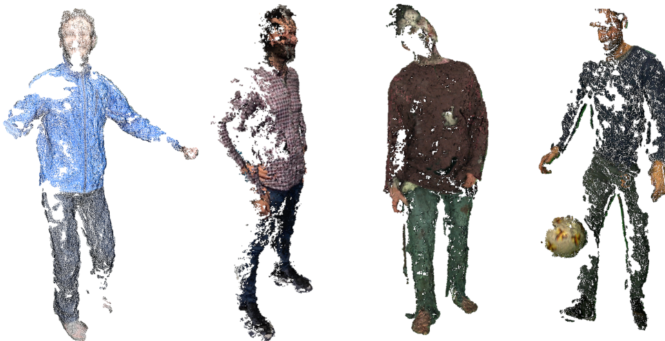
Figure 3.1: Dense point clouds generated using an affordable VV capturing platform [3]. Even after densification via multi-view stereo, the input clouds still exhibit large gaps in structure as well as patches of noise.
