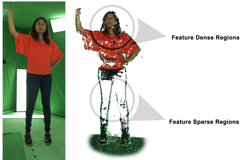
Figure 2.3: The effect of image feature richness vs feature sparsity on feature-based 3D Reconstruction
