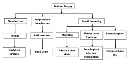
Fig. 1. A top down approach to identify the possible causes for revision of a cementless hip stem from the revision surgery, the observed failure modes, the physical mechanism associated with the failure mode and the measureable parameter associated to each failure mode (adapted from Martelli et al. (2011)).
