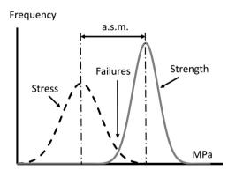
**Fig. 2.** Mechanical failure is a matter of stress versus strength, which are both distributed stochastically in a patient population. The average safety margin (a.s.m.) determines the number of failures. Adapted from Huiskes (1993).
