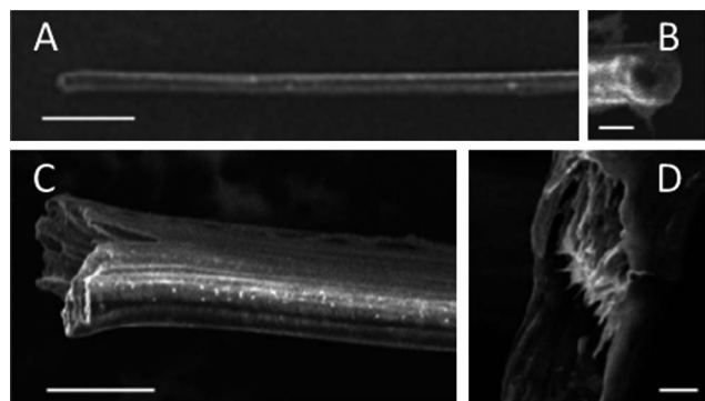
Fig. 1 SEM images of melt processed PET–SWNT fibres. The scale bars are (A) 20 \mu\text{m} , (B) 2 \mu\text{m} , (C) 10 \mu\text{m} and (D) 1 \mu\text{m} .
